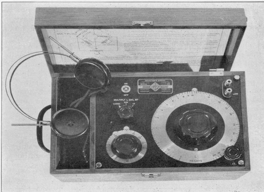
FIGURE 1. View of the TYPE 1631-A Inductance Bridge. Telephones are permanently attached to the instrument, and all necessary operating instructions are mounted in the cover. The TYPE 1614-A Capacitance Bridge is similar in appearance.
